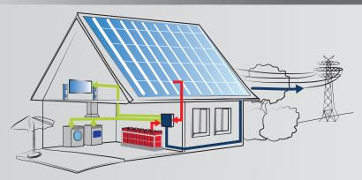
Electrical power generated by the sun and/or wind, and actual power consumption never match. The result is feedback of power into the grid when excess power is generated, and power needed from the grid when power generation is insufficient.
